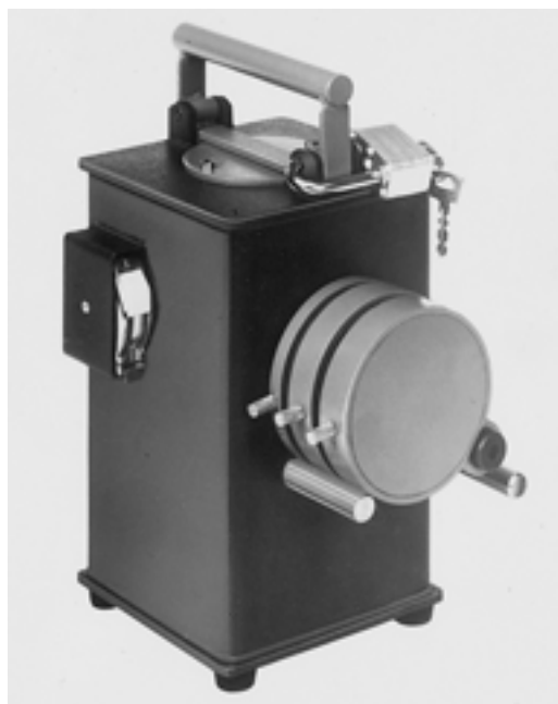
Gamma Survey Instrument Calibrator with three attenuators in place
